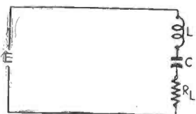
Fig. 2—The common series-resonant hookup.
